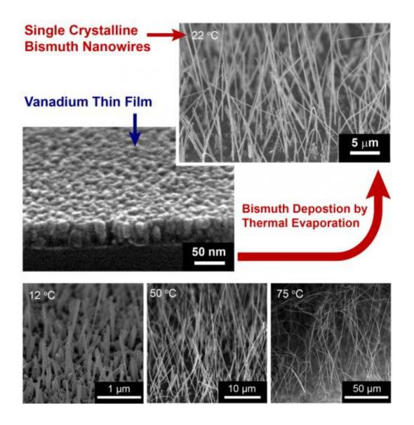
By adjusting the substrate temperature, the thickness and length of the bismuth nanowires can be tuned over very wide ranges (60-400 nm) and (1 > 100 mm), respectively.
