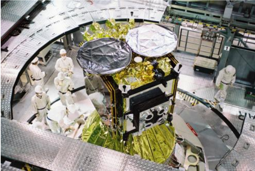
Hayabusa 2 under construction ahead of its epic journey. Credit: JAXA
