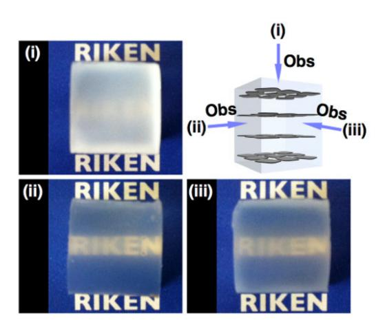
The word RIKEN is seen through the material in the orthogonal (i) and parallel (ii, iii) directions to the magnetically oriented TiNS plane.
