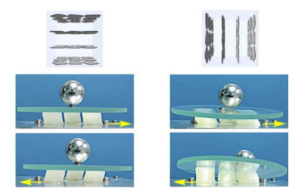
On a mechanical oscillator, a glass stage featuring a metal sphere on a tee was supported by three cylindrical pillars of magnetically structured hydrogel containing cofacially oriented TiNSs (0.8 wt%) in parallel (g) or orthogonal (h) direction to the cylinder cross-section.
