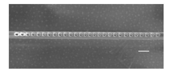
A scanning electron microscope image of the diamond photonic cavity shows the nanoscale holes etched through the layer containing NV centers. The scale bar indicates 200 nanometers. Credit: Evelyn Hu/Harvard
