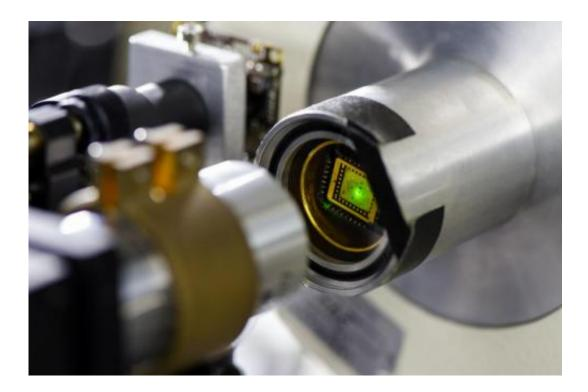
Laboratory set-up measuring the interaction between graphene and nanodiamonds with implanted nitrogen-vacancy centers. Credit: Astrid Eckert / TUM
