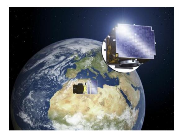
Proba-3's pair of satellites will be in a highly elliptical orbit around Earth, performing formation flying manoeuvres as well as scientific studies of the solar corona. The occulter satellite will have solar panels on its Sun-facing side. Credit: ESA - P. Carril, 2013
