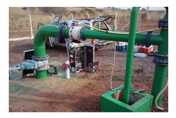
A groundbreaking Nature Geoscience article co-authored by UD geochemist Neil Sturchio describes a new method to accurately date groundwater. Pictured at a well in Brazil is machinery used for the extraction of dissolved gases from groundwater. The apparatus extracts the gases as the water flows through and compresses them into a small aluminum cylinder.
