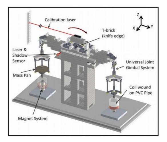
CAD model of the LEGO watt balance. The balance pivots about the T-block at the center. Two PVC endcaps with copper windings hang from universal joints off either side of the balance beam. Coil A is on the left and Coil B is on the right. A 10 gram mass sits on the Coil A mass pan and each coil is concentric to its own magnet system. Two lasers are used to calibrate and measure the linear velocity of each coil. Credit: arXiv:1412.1699 [physics.ins-det]
