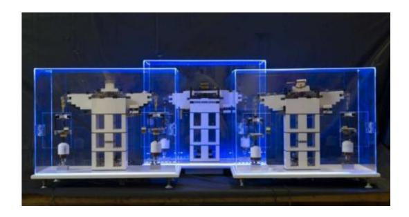
Image of three similar versions of the LEGO watt balance. The acrylic cases are backlit with blue LEDs and serve the purpose of blocking out disturbances from air currents. Two hinged doors on the front panel allow for small masses to be placed and removed from the mass pans. All the electronics are mounted below the wooden base board. Four adjustable feet are used for leveling the balance. Credit: arXiv:1412.1699 [physics.ins-det]
