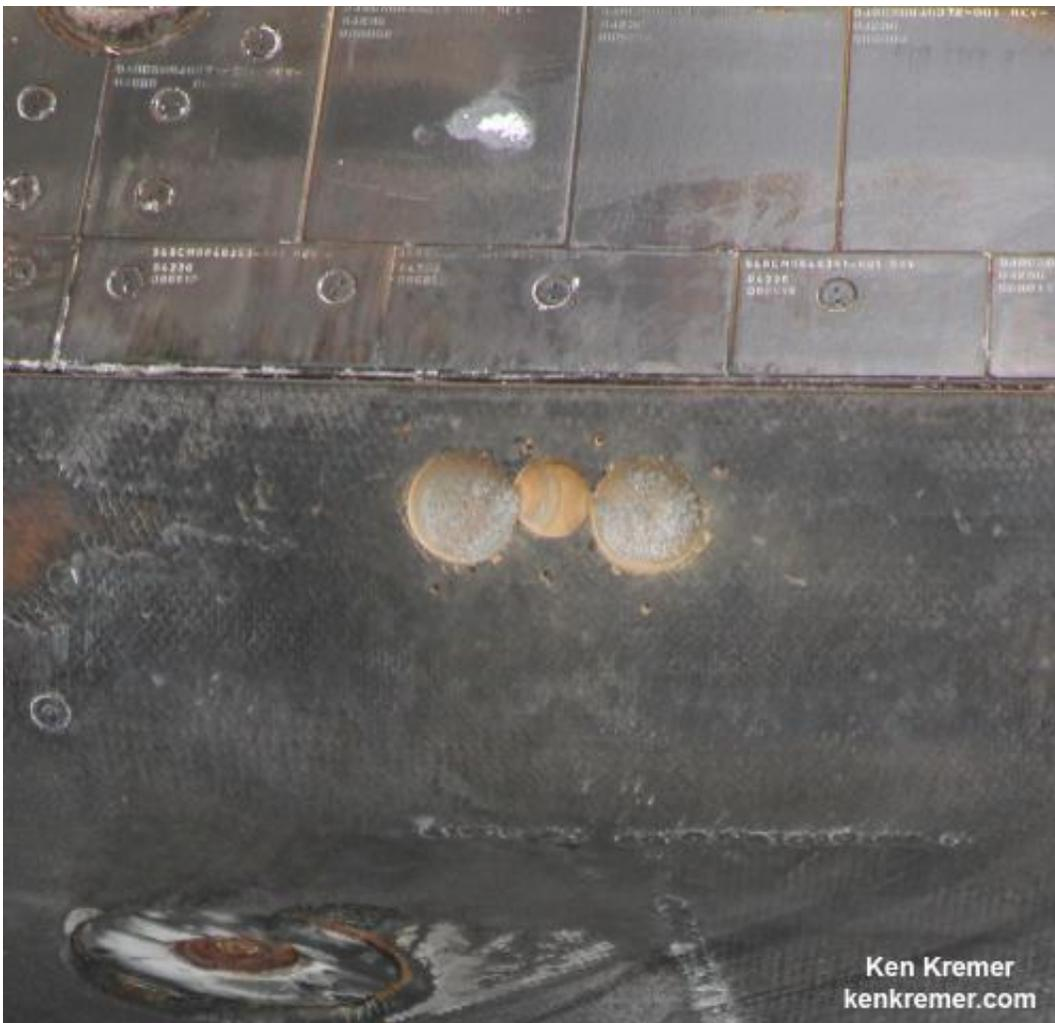
Up close view of three core samples taken from the heat shield of NASA's first Orion spacecraft after returning to NASA's Kennedy Space Center in Florida on Dec. 19, 2014. Credit: Ken Kremer – kenkremer.com
