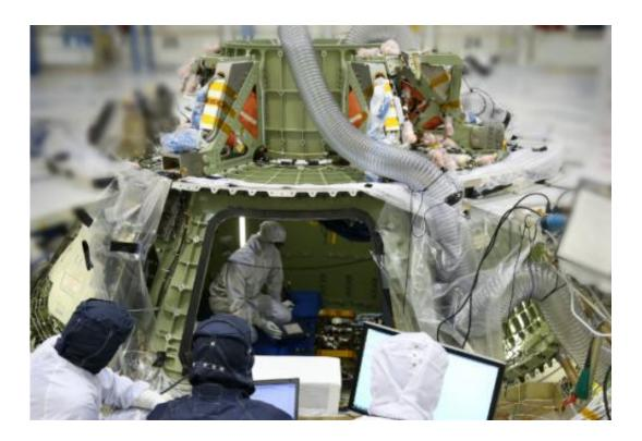
Orion's avionics system was installed on the crew module and powered up for a series of systems tests at NASA's Kennedy Space Center in Florida last week. Credit: Lockheed Martin.
