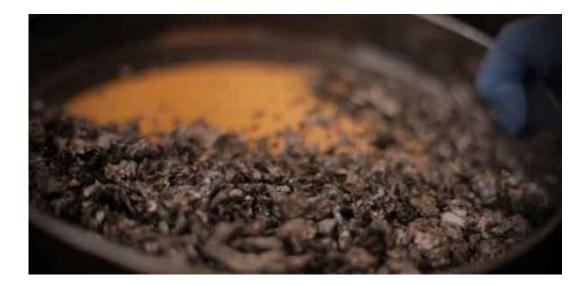
Technology developed at the University of Cambridge lies at the heart of a commercial process that can turn toothpaste tubes and drinks pouches into both aluminium and fuel in just three minutes.
