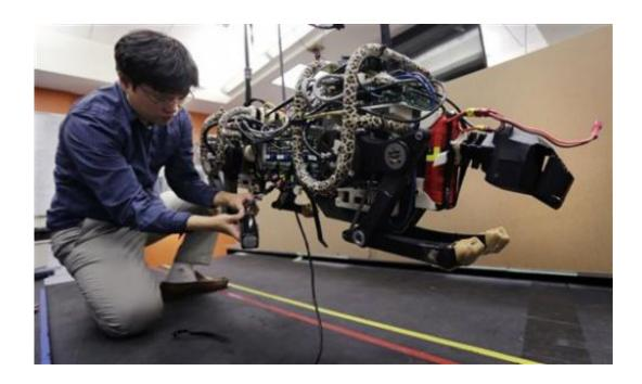
In this Sept. 30, 2014 photo, researcher Hae Won Park plugs the batteries into a robotic cheetah at the Massachusetts Institute of Technology in Cambridge, Mass. MIT scientists said the robot, modeled after the fastest land animal, may have real-world applications, including for prosthetic legs. (AP Photo/Charles Krupa)
