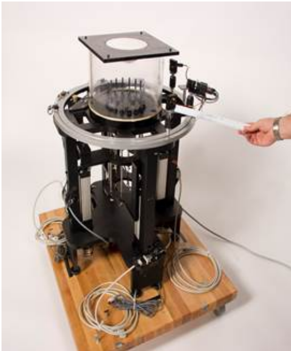
This image shows an image of a microwave breast tomography instrument. Credit: N.Epstein/U.Calgary
