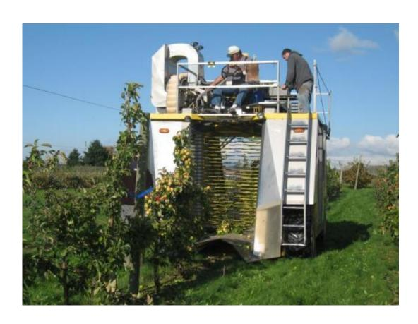
Mechanical harvest of with an over-the-row small fruit harvester was determined to be effective for harvesting cider apples. Credit: Photo by Carol Miles.
