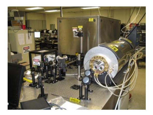
This powerful one-ton laser, capable of firing dozens of pulses a second, gives researchers a new way to detect tiny amounts of hazardous gases from up to one kilometer away, and under normal atmospheric pressure -- something that wasn't thought possible before. Credit: Henry Everitt, U.S. Army and Duke University.
