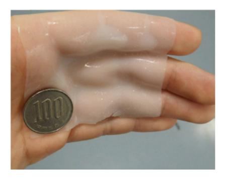
Adhesive gel with superior biocompatibility that can form patterns with light This novel type gel can follow the shape of fingers when applied to a hand. The gel surface has strong adhesion, and a 100 yen coin does not fall off by shaking.
