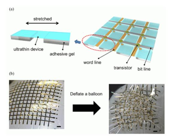
New Sheet-type Sensor. Sheet-type sensors are made by forming an adhesive gel pattern only on the electrodes after an organic transistor integrated circuit is made on an extremely thin polymeric film. The sensors did not break even after they were affixed to a balloon and 100% compression was applied.
