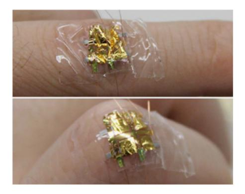
Strain sensor applied to a human finger. The strain sensor is thin and flexible and can be comfortably applied to a finger. It will not peel off or break even if great stress such as finger movement is applied.
