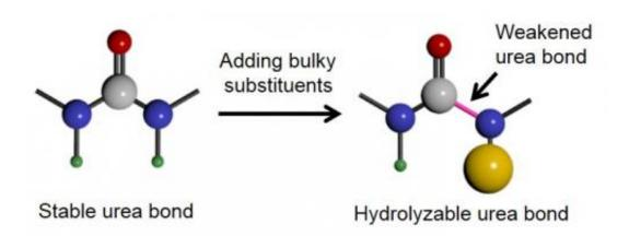
Hindered urea bond-containing polymeric materials (PHUs) are cheap polymers that can be designed to degrade over a specified time period. Credit: Catherine Yao
