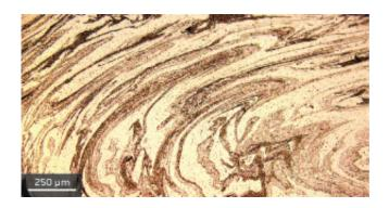
Scanning electron micrograph showing the complex flow patterns, or 'onion rings', formed on the advancing side of the welding tool. Credit: A\*STAR Singapore Institute of Manufacturing Technology
