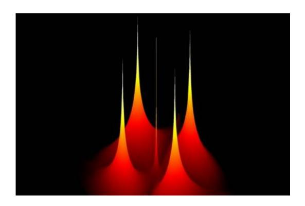
Plot of radiative quality factor as a function of wave vector for a photonic crystal slab. At five positions, this factor diverges to infinity, corresponding to special solutions of Maxwell equations called bound states in the continuum. These states have enough energy to escape to infinity but remain spatially localized.
