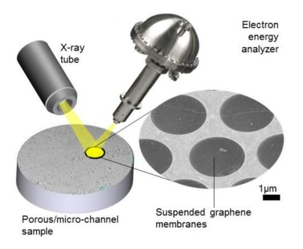
Drawing shows the set-up for an X-ray photoelectron spectroscopy instrument incorporating suspended, electron-transparent graphene membranes—or windows—that separate the sample from the high-vacuum detection system. Credit: NIST
