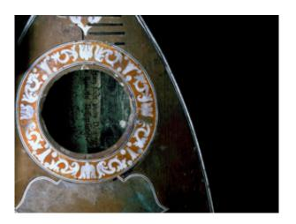
Fluorescence induced by ultraviolet radiation of a mandolin made by G.Filano, particularly of the sound hole decoration. The orange color is characteristic of the resin of the false inlay, which organic fraction seems to be composed by shellac only. © Rovetta/Canevari
