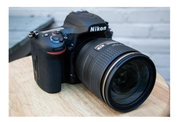
This Dec. 16, 2014 photo shows the Nikon D750 camera, in Decatur, Ga. The D750 is a full-frame digital SLR camera capable of shooting high-definition video at 60 frames per second. It has a 24.3 megapixel sensor and built-in Wi-Fi for communication directly with tablets and smartphones. (AP Photo/Ron Harris)
