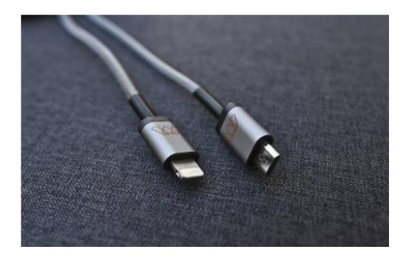
This Wednesday, Dec. 10, 2014 photo shows the MOS smartphone charging cables, in Decatur, Ga. The cables are reinforced with strong woven material along their length and anodized aluminum protection at the connector ends. (AP Photo/Ron Harris)
