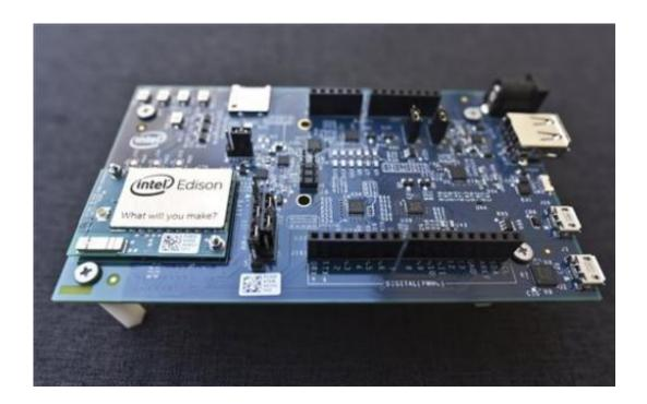
This Wednesday, Dec. 10, 2014 photo shows the Intel Edison, a small programmable computer the size of an SD memory card, seated on an electronics expansion board, in Decatur, Ga. The Edison has both Wi-Fi and Bluetooth technology built in, as well as a full distribution of the Linux operating system. (AP Photo/Ron Harris)
