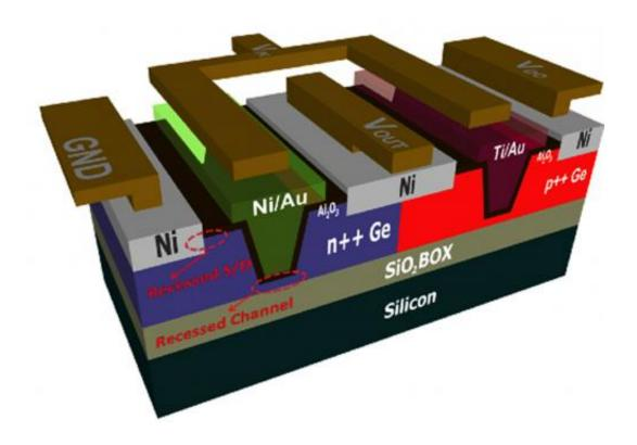
This graphic depicts a new electronic device created at Purdue that uses germanium as the semiconductor instead of silicon. Germanium is one material being considered to replace silicon in future chips because it could enable the industry to make smaller transistors and more compact integrated circuits. Credit: Purdue University image
