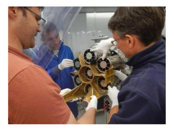
Installing state-of-the-art optics onto the Focusing Optics X-ray Solar Imager, or FOXSI, mission, which will observe hard X-rays from the sun. Credit: NASA/FOXSI
