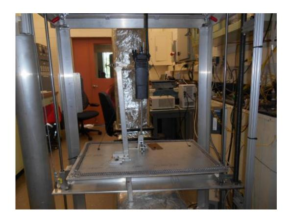
A portable firefighter radio is instrumented for testing in a NIST-designed apparatus that consistently creates thermal conditions representative of typical fire environments. Data and performance measurements recorded with the equipment are furnished to the National Fire Protection Association, which is developing a performance standard for portable radios used by emergency personnel. Credit: NIST
