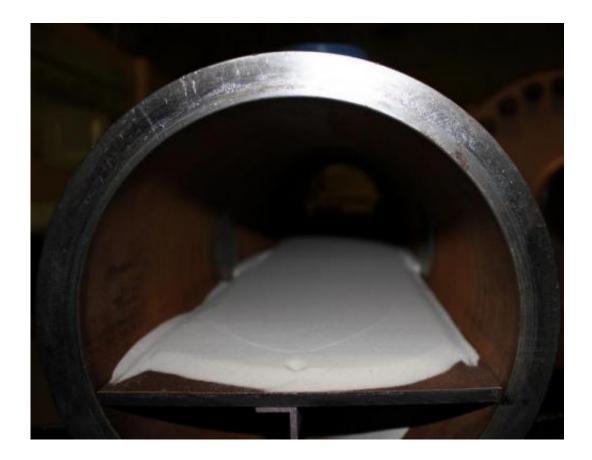
Sediment inside the Titan wind tunnel for testing. Credit: University of Tennessee
