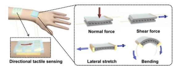
Touch can be a subtle sense, but it communicates quickly whether something in our hands is slipping, for example, so we can tighten our grip. For the first time, scientists report the development of a stretchable "electronic skin" closely modeled after our own that can detect not just pressure, but also what direction it's coming from. The study on the advance, which could have applications for prosthetics and robotics, appears in the journal *ACS Nano*.
