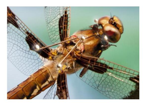
This is a composite image of dragonfly carrying retroreflective markers. The markers are used to measure the orientation of the dragonfly's head and body during flight. The data from the measurements allows the underlying steering strategy to be inferred. Credit: Igor Siwanowicz, Leonardo Lab, HHMI/Janelia Research Campus
