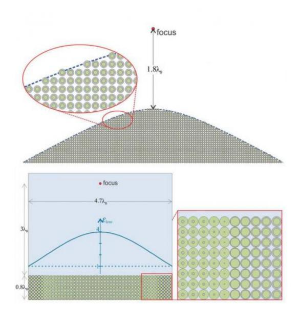
A metamaterial with a given permittivity can be designed out of any two materials, called 'metamaterial bits,' so long as the permittivity of one of the
