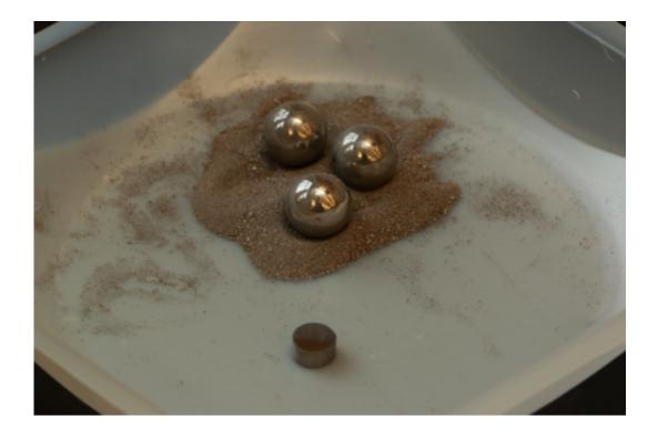
A compacted metal alloy pellet sits next to as-milled tungsten-chromium iron metal powders in a boat used for weighing the metals. The steel balls are used to deform the metals in a high-energy ball mill. Credit: Denis Paiste/Materials Processing Center
