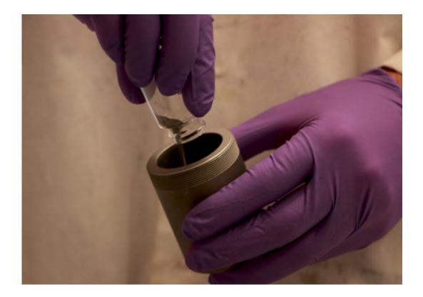
Zack Cordero pours tungsten-chromium iron powder into a steel vial used to deform the metal in a high-energy ball mill. The deformation process, which involves repeated shearing of the metal powders, drives the alloying elements to intermix creating an exceptionally strong nanostructure. Credit: Denis Paiste/Materials Processing Center
