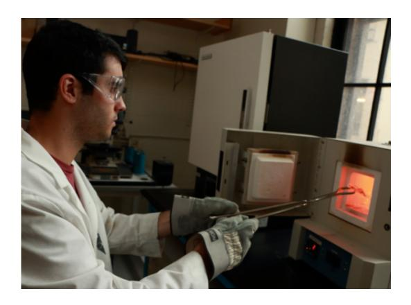
MIT graduate student Zack Cordero removes a vacuum-sealed glass ampoule from a box furnace operating at 1,100 degrees Celsius that is used to anneal metal powders. Credit: Denis Paiste/Materials Processing Center
