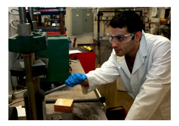
MIT graduate student Zack Cordero demonstrates a uniaxial press used for consolidating loose powder into a pellet. Working under Materials Science and Engineering Department chair Christopher A. Schuh, Cordero has developed extremely hard, finely grained tungsten alloy powders and compacts. Credit: Denis Paiste/Materials Processing Center
