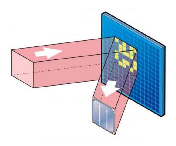
Patterns of light are projected onto PV cells to measure their response
