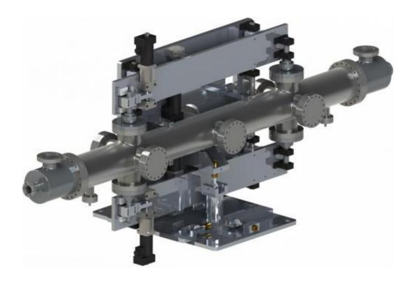
Design drawing of the outer structure of a dechirper that will be used to tweak the "color range" of light pulses from SLAC's X-ray laser, LCLS. Two dechirpers will be lined up in front of the LCLS undulator—a magnetic structure that generates ultrabright, ultrafast X-rays from bunches of electrons. Credit: RadiaBeam Systems
