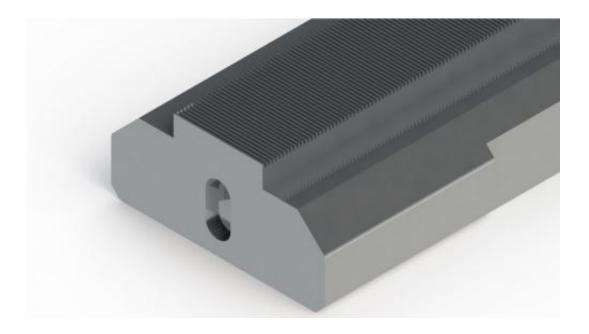
The aluminum rails have comb-like grooves that are half a millimeter deep and a quarter millimeter wide. The electron bunches "sense" the grooves, leading to a change in the energy spread of the X-rays they produce. Credit: RadiaBeam Systems
