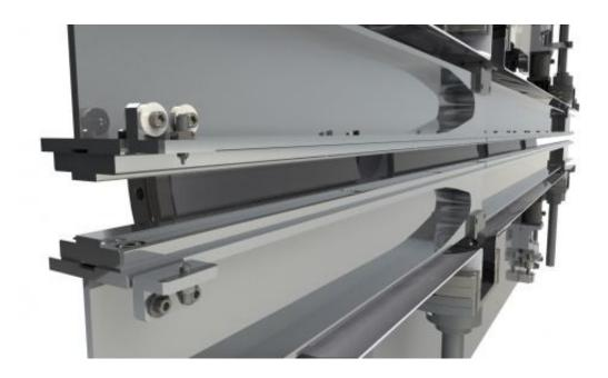
The inside of the dechirper consists of two parallel, 2-meter-long, flat aluminum rails. Electron bunches will travel through a variable gap between the rails at nearly the speed of light. Credit: RadiaBeam Systems
