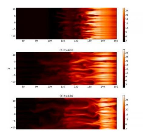
Solar snapshots: Three time-lapse excerpts from the new simulation computation based on magnetohydrodynamics. The evolution of the dark finger-like structures, which indicate the Rayleigh-Taylor instability, can be clearly seen. Credit: MPS
