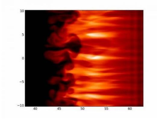
Streaming gas in the corona: Here a typical result of the new simulation computation based on magnetohydrodynamics. As in the observations, the dark finger-like structures indicate the Rayleigh-Taylor instability. Credit: MPS
