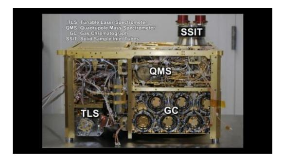
SAM's three instruments are visible in this view taken before installation of its side panels: the tunable laser spectrometer (TLS) at lower left, the quadrupole mass spectrometer (QMS) at upper right, and the gas chromatograph (GC) at lower right. Credit: NASA
