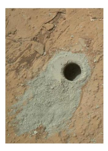
NASA's Mars rover Curiosity drilled into this rock target, "Cumberland," during the 279th Martian day, or sol, of the rover's work on Mars (May 19, 2013) and collected a powdered sample of material from the rock's interior. Credit: NASA/JPL-Caltech/MSSS
