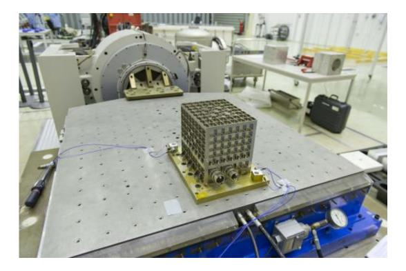
The SCCO 'Soret Coefficient in Crude Oil' experiment on the 80 kN Shaker table at ESA's test centre in Noordwijk, the Netherlands, to reproduce the extreme forces of launch and reentry. Credit: ESA–Anneke LE Floc'h
