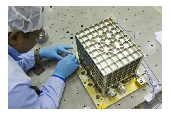
ESA's 'Soret Coefficient in Crude Oil' experiment will test diffusion effects in high-pressure crude oil. Consisting of six sturdy cylinders, each containing a millilitre of crude oil, pressurised to 400 times our normal atmospheric level, SCOO is being prepared to fly on China's SJ-10 Shi Jian spacecraft near the end of 2015, along with around 20 other experiments. Credit: ESA–Anneke Le Floc'h
