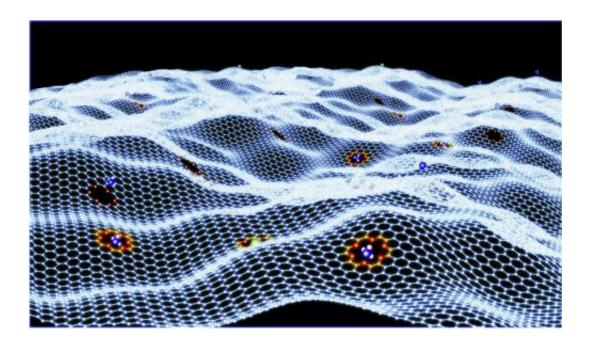
This sheet of graphene contains an array of crown ethers that can strongly bind select guest ions or molecules. Credit: Oak Ridge National Laboratory
