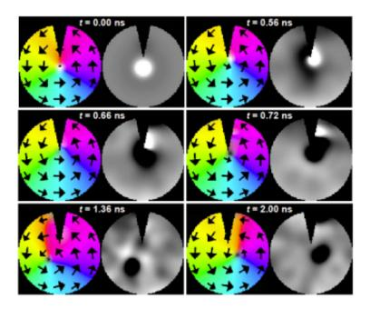
Prof. Nakatani team performed micro-magnetic simulations and took snapshots of the Pac-man disk (diameter = 200 nm, thickness = 40 nm) at different times (t =  $0 \sim 2.0$  ns). The rainbow images indicating the direction of the in-plane magnetization component, whereas the grayscale images show the out-of-plane magnetization (white,up; black,down). The vortex core switches from upward to downward.
