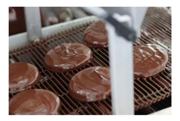
On the conveyor belt, chocolate-coated wafers are moved through the cooling channel. Credit: Fraunhofer IVV
