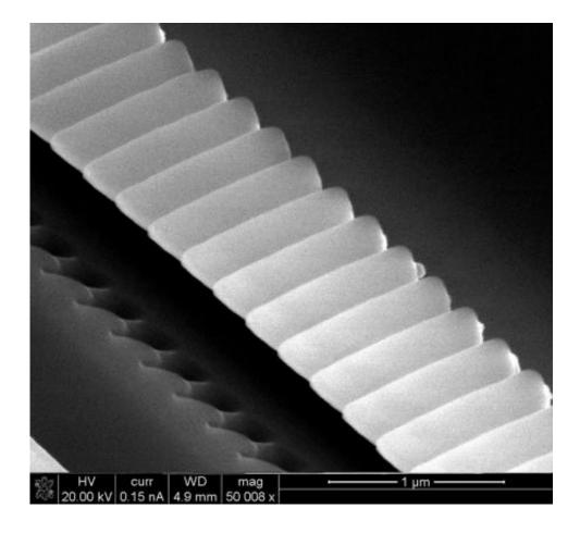
A nanoscale optical device that can be used as a quantum memory for photons. Milled from yttrium orthosilicate and doped with neodymium ions, the device (white) looks like the world's tiniest Toblerone bar. Credit: Tian Zhong/Caltech
