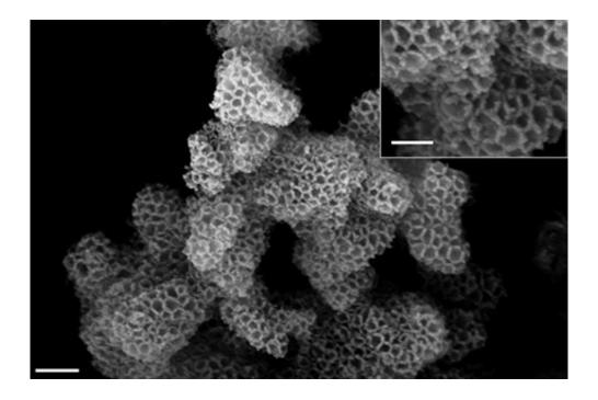
A scanning electron microscopy image of a pristine silica support, before the amine is added. Credit: Genggeng Qi
