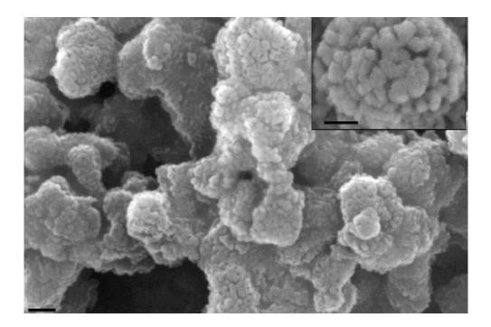
A scanning electron microscopy image of the amine sorbent. Credit: Genggeng Qi
