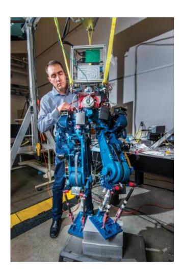
Steve Buerger is leading a Sandia National Laboratories project to demonstrate how energy efficient biped walking robots could become. Increased efficiency could enable bots to operate for much longer periods of time without recharging batteries, an important factor in emergency situations. Credit: Randy Montoya
