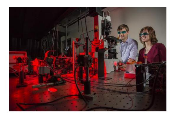
Sandia National Laboratories researchers Bryan Kaehr and Kristin Meyer analyze a silicized surface using optical microscopy and multiphoton fluorescence. Credit: Randy Montoya
