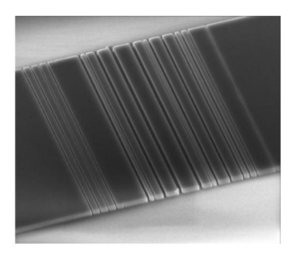
This tiny slice of silicon, etched in Jelena Vuckovic's lab at Stanford with a pattern that resembles a bar code, is one step on the way toward linking computer components with light instead of wires. Credit: Vuckovic Lab
