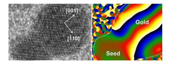
This picture combines a transmission electron microscope image of a nanodumbbell with a gold domain oriented in direction. The seed and gold domains in the dumbbell in the image on the right are identified by geometric phase analysis. Credit: Soon Gu Kwon
