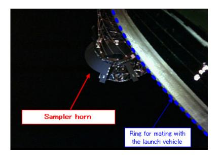
Sampler horn deployment images taken by the Hayabusa2 onboard monitoring camera thanks to your donations.
