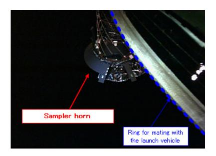
Sampler horn deployment images taken by the Hayabusa2 onboard monitoring camera thanks to your donations.
