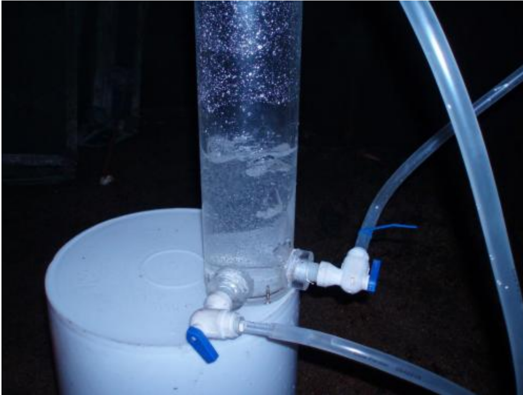
Sampling equipment to measure flow rates for fracture waters. Credit: B. Sherwood Lollar.
