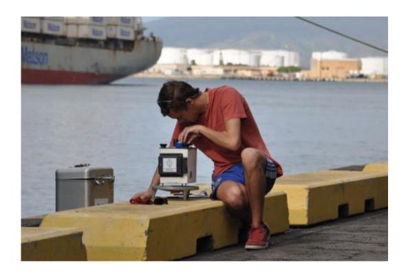
Before leaving port, an undergraduate student acquires important control data (on-shore gravimetrics) using a gravitometer. Credit: Aric Velbel, Jurassic Magnetism
