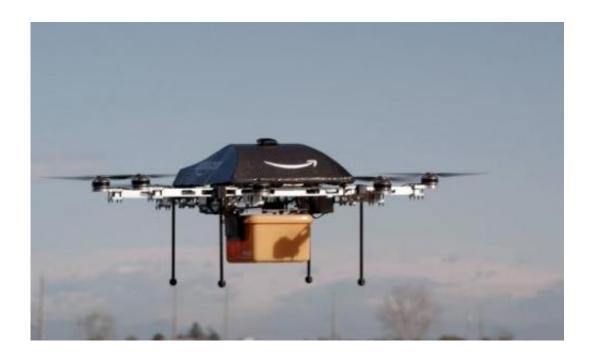
An Amazon flying "octocopter" mini-drone that could be used to fly small packages to consumers
